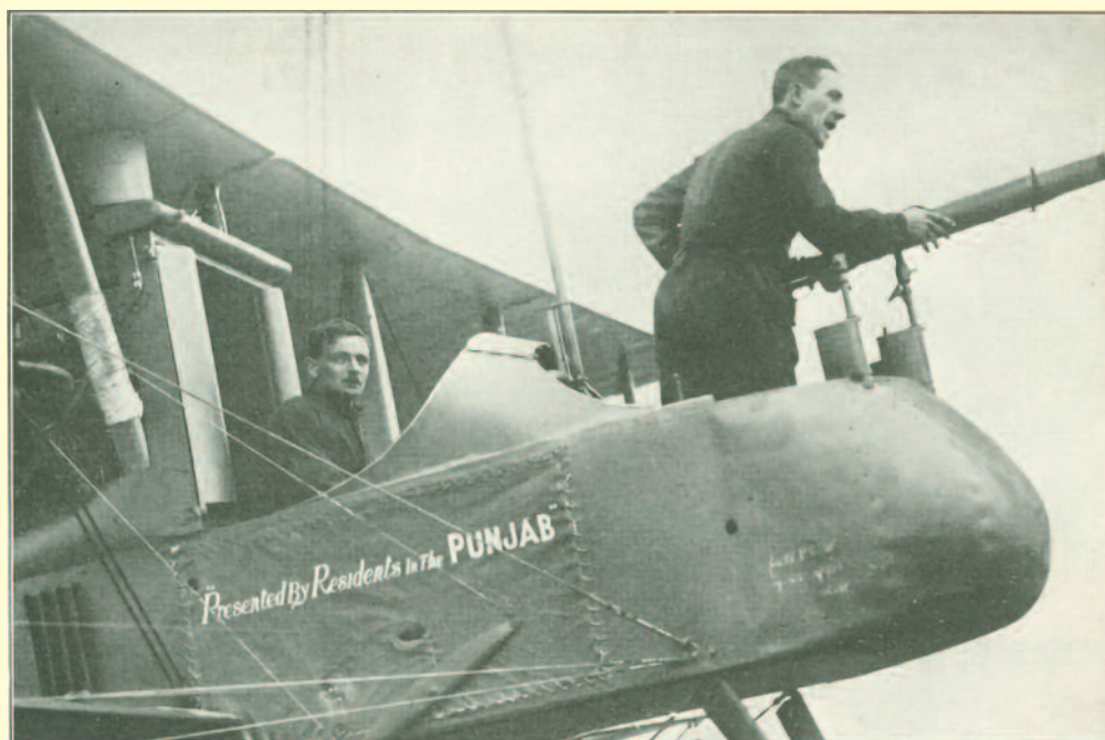
Early fighter planes are called Pushers because the engine and propeller are behind the crew and gun
